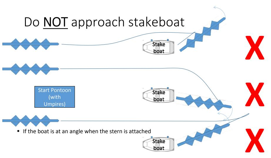
• The stream and the wind will turn the boat more quickly than you can straighten it
